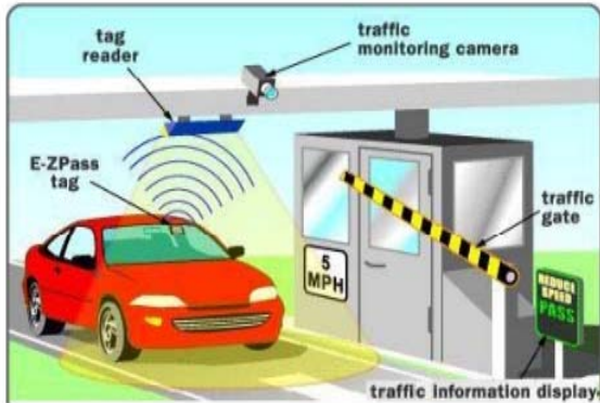
Fig. 7. Construction of Toll Plaza of System in Paper[3]
